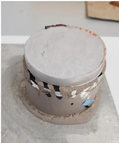
Figure 3: Left, Wet concreted poured on the wires. Right: Change in the resistance of wires as a function of time, after pouring the concrete.
